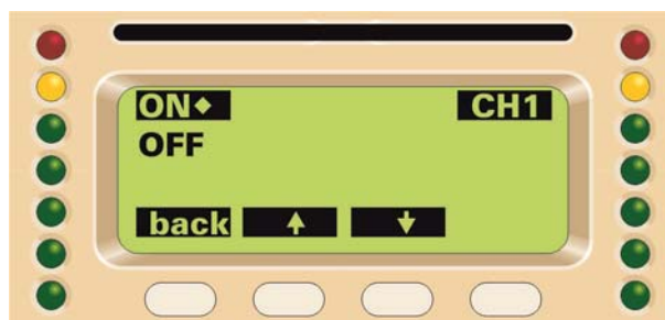
Edit CH1, go to LP Filter, set Active=ON
